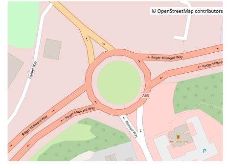
Highways England had planned significant improvements to the A63 Roger Millward Way roundabout in Hull (Figure 1), which would see it converted from a conventionally signalised roundabout to a signalised hamburger.
