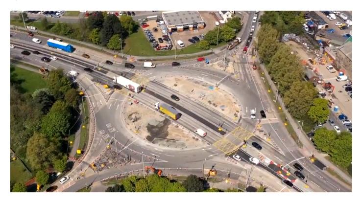
A second significant conclusion can be drawn: The SRL Urban64 signals can successfully operate MOVA control, and the benefits typically released with MOVA control of intelligent, adaptive control are now available on these temporary signals. [The 'teething troubles' on this project are expected to be a one-off and are now fully understood and resolved.]
